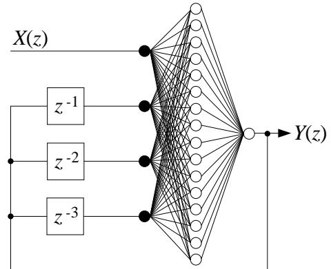
Fig. 5. Multilayer neural network NEWFF structure.
