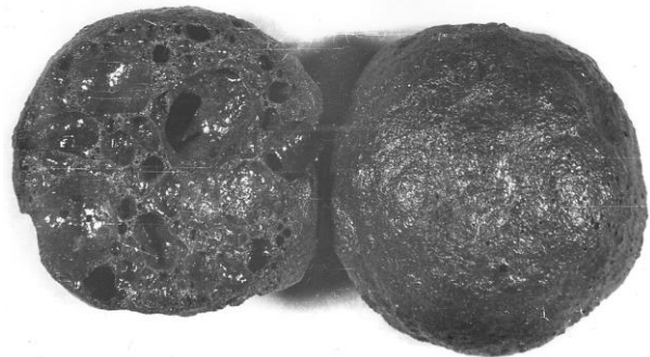
Fig. 9. General view of aggregate granules, d=25 mm.
