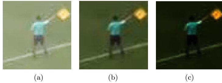
Fig. 3. Impact of the gamma correction on the illuminance of an input image. (a) \gamma = 0.5 , (b) \gamma = 1.0 , (c) \gamma = 2.0
