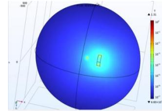
Fig. 5. The distribution of the magnetic field strength in the cross section with the Y-axis:
