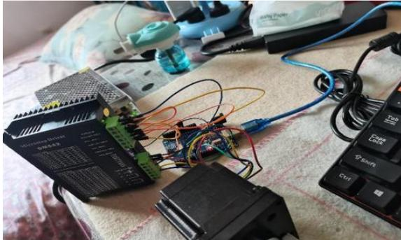
Fig. 13. Stepper motor controller and arduino wiring
