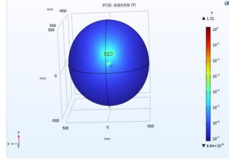
Fig. 3. The distribution of the magnetic field strength in the cross section with the Z-axis;
