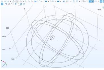
Fig. 2. The larger cylinder is an electromagnet, the smaller one is a NdFeB magnet, the ring around the electromagnet represents infinite space.
