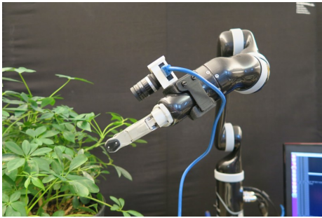
Fig. 7: Experimental setup to determine the effectiveness of the leaf acquisition algorithm. In this setup, the camera begins in a position roughly the same distance to the plant as it would in a field test.
