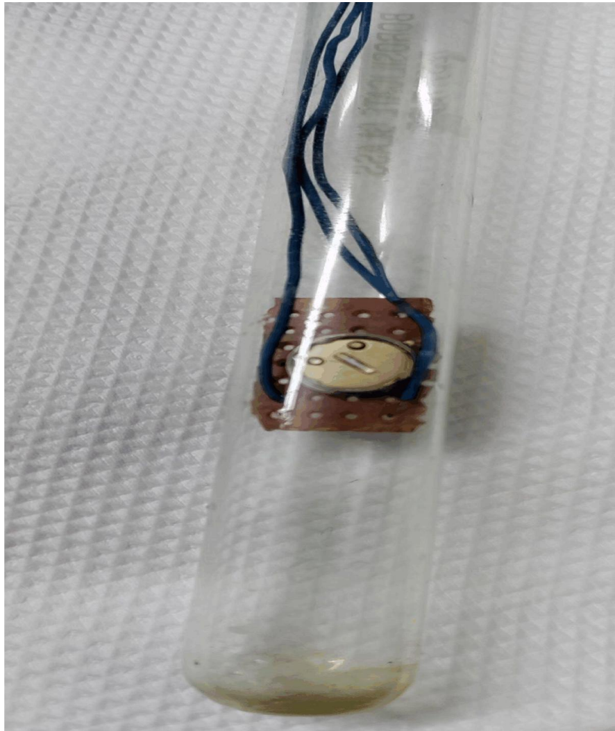
Figure 9: A SAW temperature sensor put in the test tube
