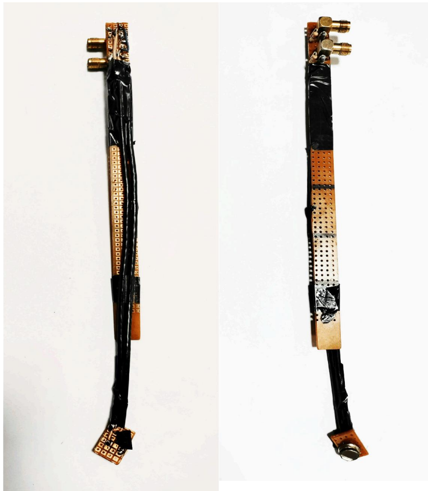
Figure 8: A SAW sensor zig with SMA connector (a) front view (b) back
