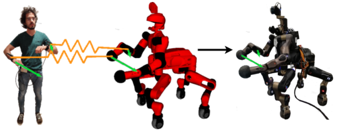
Fig. 2. The TelePhysicalOperation concept resembles a “Marionette” interface: through virtual springs, the operator applies virtual forces on the selected robot body parts, and the robot will generate compliant motions.
