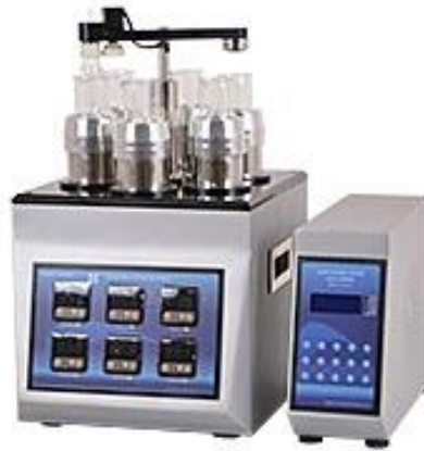
Figure 6. The SILAR controller Coating with Stirrer.
