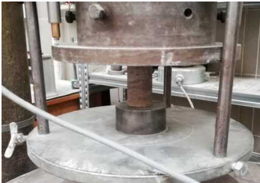
Figure 1: Uniaxial compressive test
