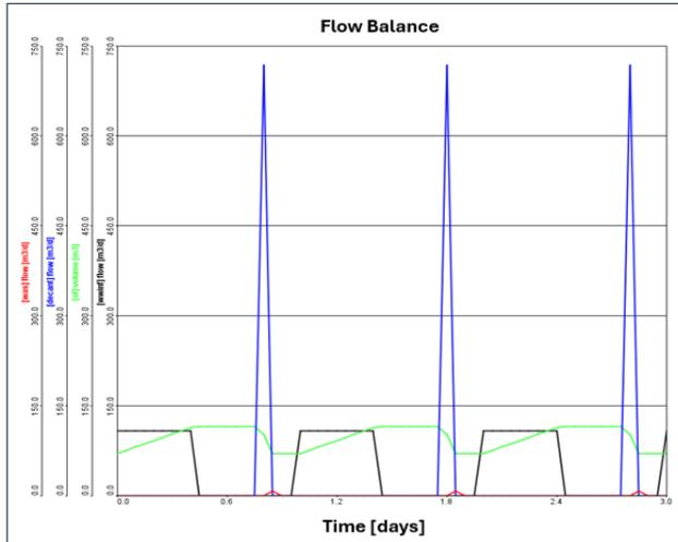
Fig. 4 The simulation environment in GPS-X with the influent and effluent flow balance of the simple SBR model. The plotted black line is the influent flow, the blue plotted line being the effluent (decant) flow and the red plotted line is the sludge waste flow. The green line is the hydraulic volume of the SRR.
