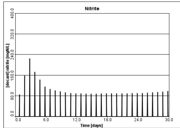
Fig. 9 Simulation of the effluent concentration of nitrite [mgN/L] in the advanced SBR model. Simulation was done at DO setpoint of 1.5 mg/L.
