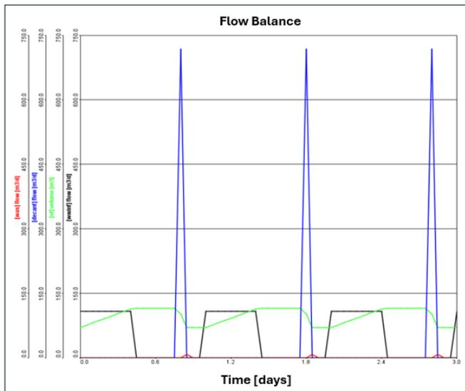
Fig. 7 The flow balance of the advanced SBR model. The black line is the influent flow, the blue line is the decant flow and the red is the waste flow. The green plotted line shows the hydraulic volume of the reactor.
