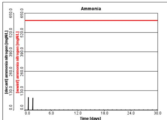
Fig. 8 Simulation of ammonia removal in advanced SBR model. The constant influent concentration of ammonia (red line) and the effluent ammonia concentration (black). Simulation was done at DO setpoint of 2.0 mg/L.
