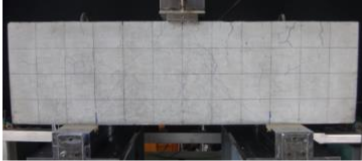
Fig.2 The picture of specimen after cracking
