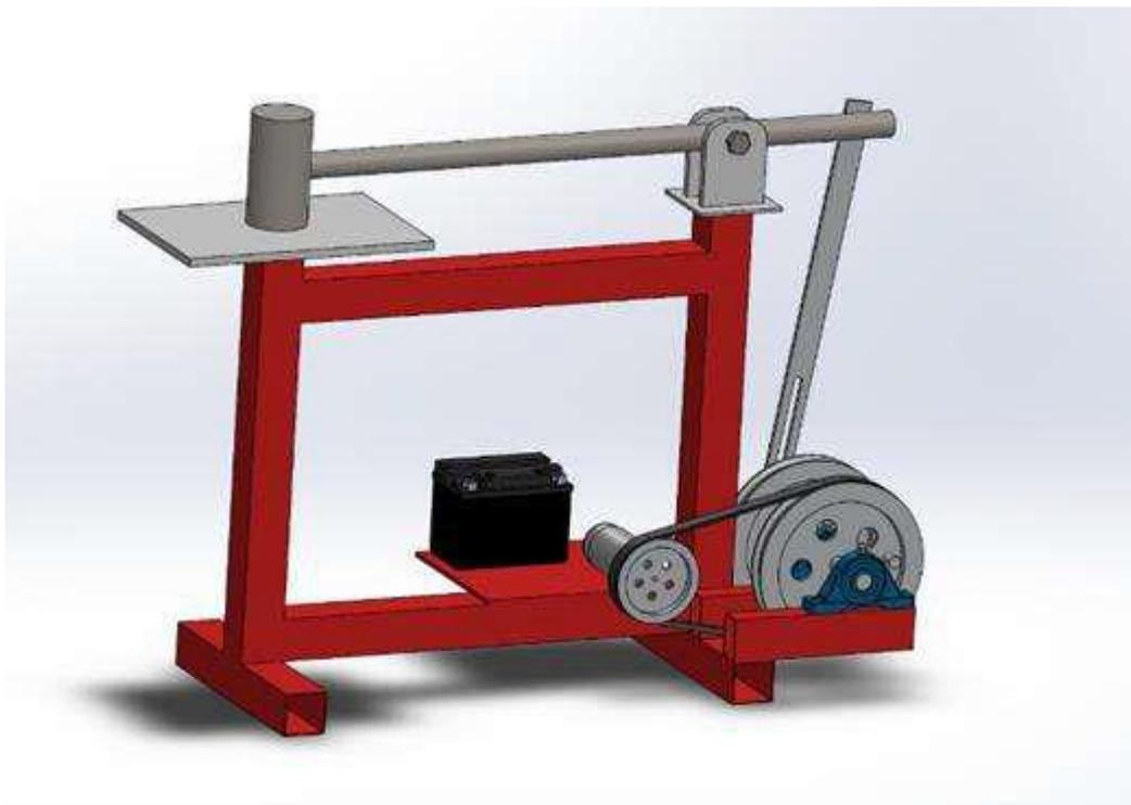
Figure 1.1.2 Simple Electric Hammering Machine
