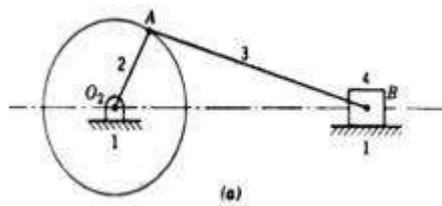
Figure 1.1.3 Slider Crank Mechanism
