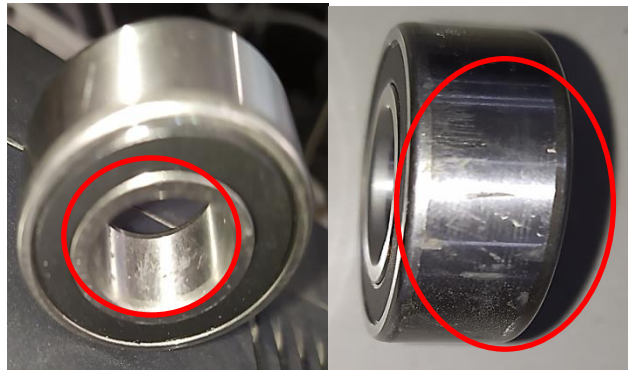
Fig.2. Bearing with inner race and outer race defects used in the experimental tests
