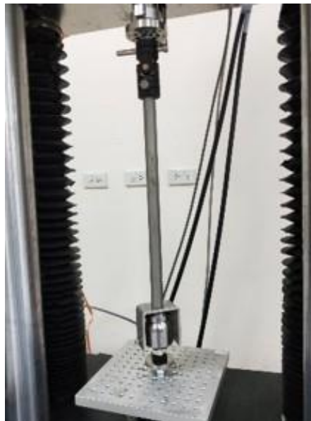
Fig. 3 Dynamic axial compression fatigue test fixture
