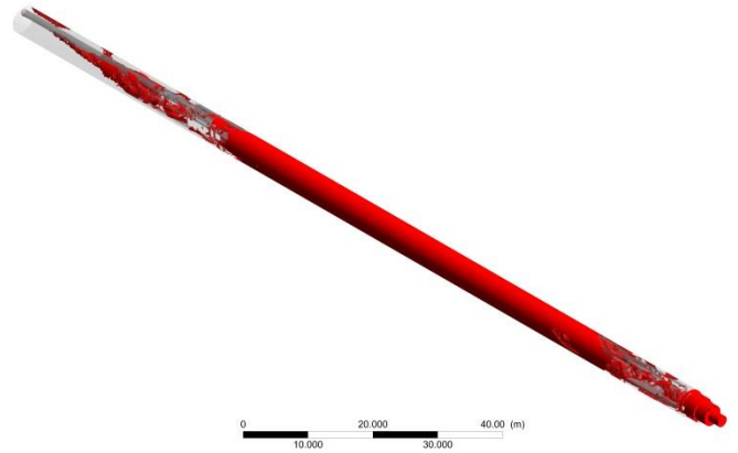
Figure 4 Dead zone volume in switch off exhausting fan scenario
