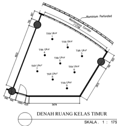
FIGURE 5. Classroom measurement points with east oriented
