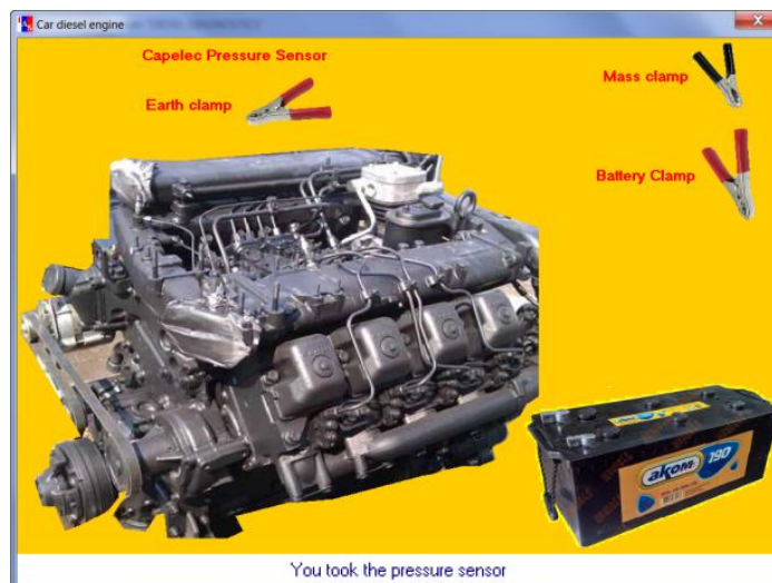
Fig. 3. Window with connection points of primary converters to the engine
