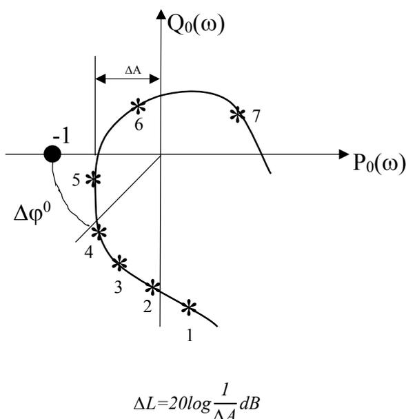
Fig. 6. Amplitude-phase characteristics of the "open" system of the machine adopted into the automation system.
