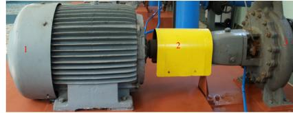
Fig. 3 - View of the tested machine (1 - engine, 2 - coupling, 3 - pump).
