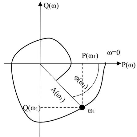
Fig. 2. Amplitude-phase characteristics in the rectangular  $P$  and  $Q$  coordinates and the polar  $A$  and  $\varphi$  coordinates.
