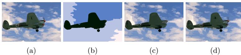
Fig. 1: (a) Original image and its segmented version for (b) 4, (c) 128 and (d) 256 superpixels.
