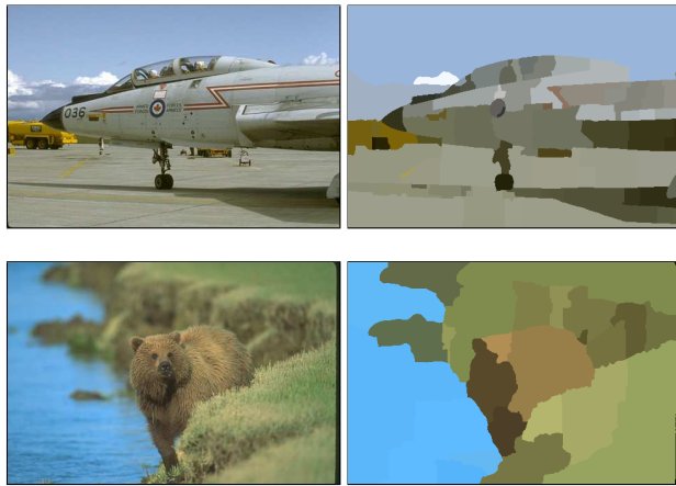
Fig. 3: Examples of SH result with number of superpixels defined automatically by Mean Shift over the hue version of the images. Original images are presented in the left column and their respective superpixel versions are in the right column.
