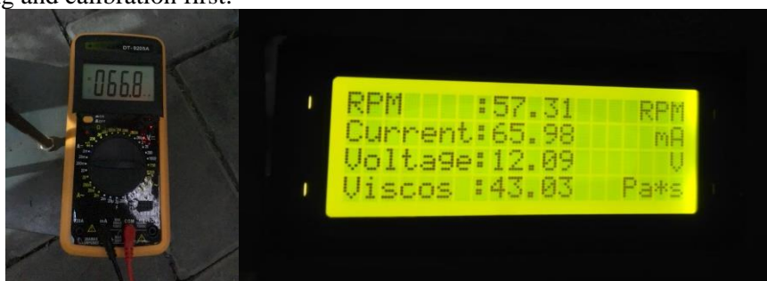
Figure 10. DC motor current test
