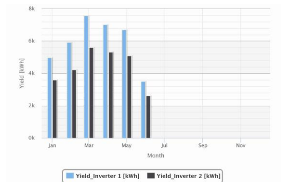
FIGURE 8: Yield of 100 kW SPV Power Plant for year 2018 Figure 8 shows the yield of 100 kW Solar photo voltaic (SPV) Power Plant for year 2018. Maximum yield has been achieved in the month of March 2018.
