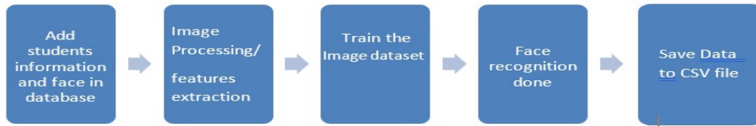
Fig 4.1 Flow chart for Integrated Student Database and Attendance Management System with Face Recognition
