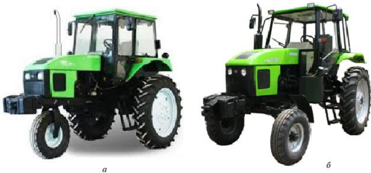
Figure 1. Universal-tiller tractors with 3W2 (a) and 4W2 (b) wheel arrangements
