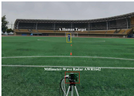
Fig. 3. The experimental environment: A human target straightly moves away from AWR1642 radar with constant velocity 1.3m/s.
