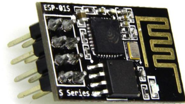
Figure 5. ESP8266 wireless communication module
