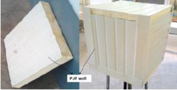
Fig. 3, (a) Insulating PUF wall (b) Insulating test cabin
