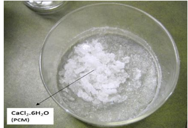
Fig. 1 Crystal foam of \text{CaCl}_2 \cdot 6\text{H}_2\text{O} in the biker.
