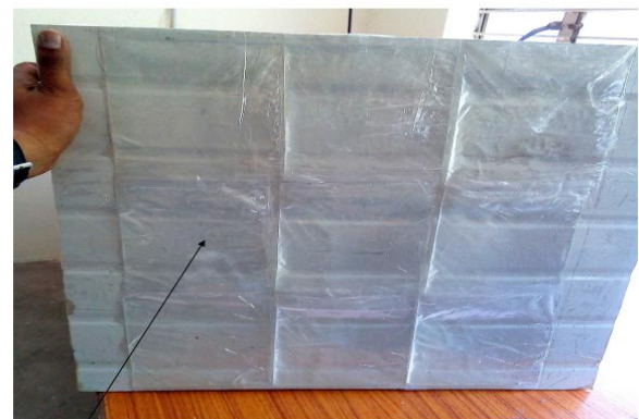
Fig. 2 PCM augmented composite wall.
