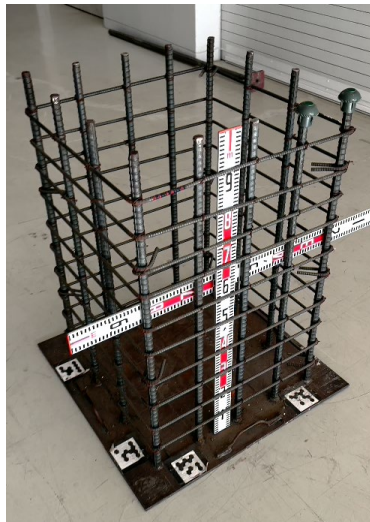
Figure 4: Target sample of the rebar cage)
