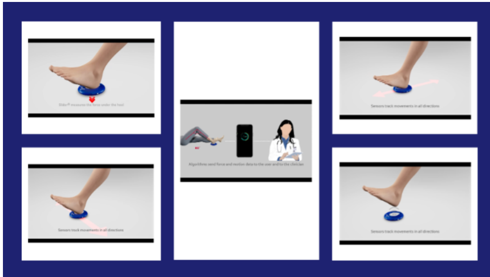
Figure 1 - Slider measures force and tracks movements in all directions. It sends data to the user's tablet and to the clinician.
